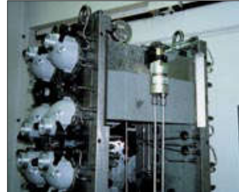
■ PID-Series intensifier utilizes low pressure machine hydraulics to power clamping cylinders.
