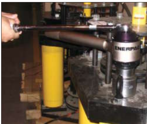
◀ Enerpac E393 Torque Multiplier used to manually torque bolts up to 3,200 ft. lbs.
