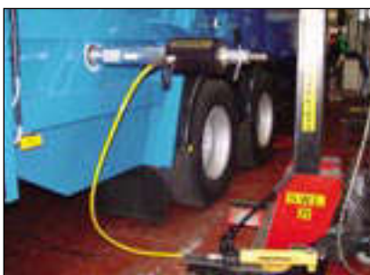
◀ An RACH-606 powered by a P-392 handpump used to extract corroded carriage pins of refuse collection vehicles.
